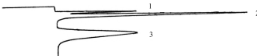
Figure 2 Chromatogram of the separation of aniline derivatives on C 18 -PBD-ZrO 2
